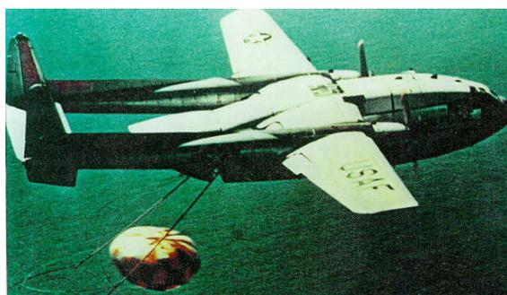
**Figure 2. The parachute (yellow) carrying a CORONA capsule with its undeveloped film is snared by the catcher plane over the Pacific Ocean**
