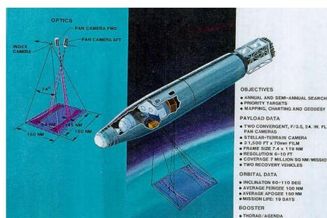
**Figure 1. Typical CORONA stereo camera configuration built on the Agena upper stage**
